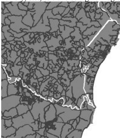
Figure 1. Image of a trafficability map of the Itaoca, ES region for troops on foot during the day with dry weather. Darker colors represent lower costs (roads). The white color represents an untraversable region (the sea and some rivers).
