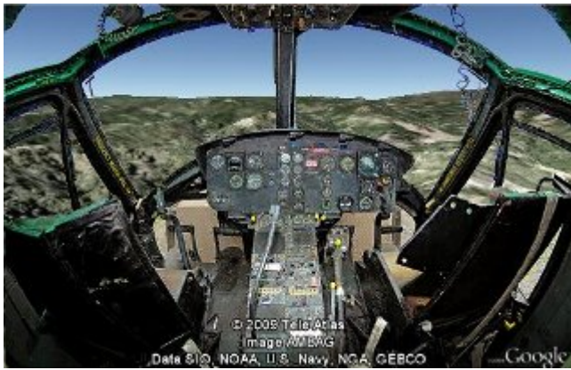
Figure 1: The aerial reconnaissance system using Google Earth API to display a raster image with transparent helicopter cockpit above the Google Earth terrain
