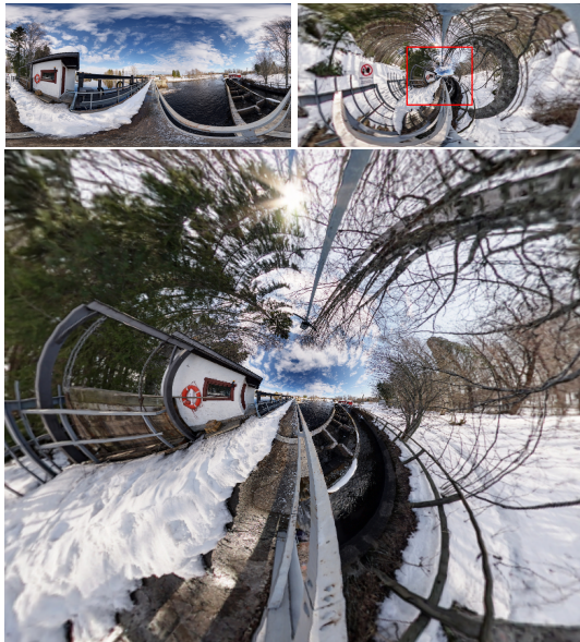
Figure 5: Top-left: input equi-rectangular image. Top-right: result of applying a scale s = 0.05 on the viewing sphere. Bottom: result of perspective projection applied to the transformed viewing sphere (showing only the area inside the red rectangle of the top-right figure). Although almost the entire viewing sphere is being shown, unpleasant straight line distortions appear.
